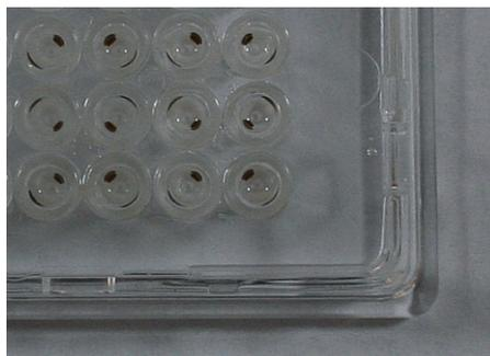
***Magnetic Beads are pulled to the sides of each well***
